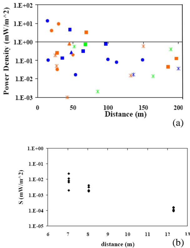
Figure 1: Measured GSM-900 peak power density levels as a function of distance to the nearest base station (derived from [3]) (a). For comparison, WLAN peak power density levels as a function of distance to the nearest WLAN router ([4]) (b).
